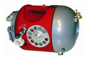
The **Model K** pull type Lasher handles just about any size lashing job. Use it to single- or double-lash a single cable up to 3 1/2" outside diameter and multiple cables up to a combined outside diameter of 4 5/8".
