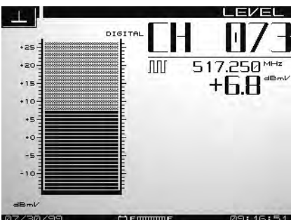
Digital channel average power measurements can be made using the digiCheck™ feature
