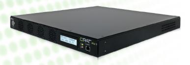
As soon as the digital test signal pilot is detected at the input of the IRX1, its data is decoded. The vehicle ID, event time stamp and RF level are then recorded. The IRX1 stores and communicates upstream decoded data back to the CPAT server, through the 10/100 BaseT Ethernet connection. With the IRX1's high capacity processing power, there is no limit to the number of vehicles that can be equipped with an ITX1 transmitter module.
