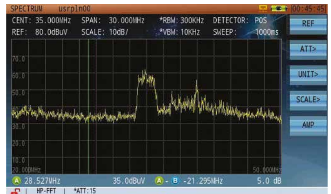
Figure 4: Spectrum Analysis: Traditional view of the upstream spectrum noise covered by signal.
