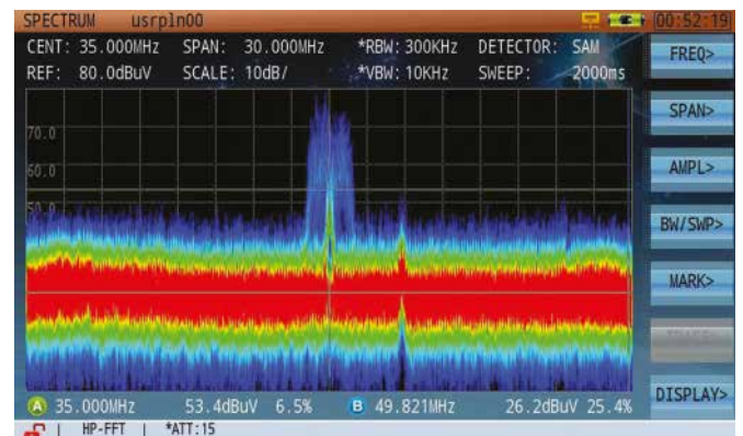
Figure 5: Persistence Technology Shows Ingress Signal Under DOCSIS Upstream Signal
