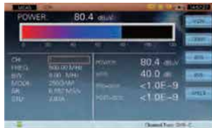
QAM signal quality measurement
