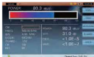
DVB-T signal measurement
