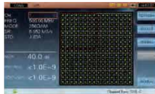
QAM constellation measurement
