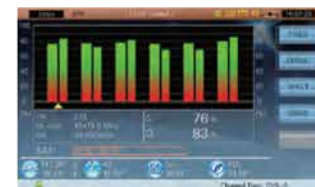
Display Max. 12 Transponder Signals' quality to Align DishAntenna
