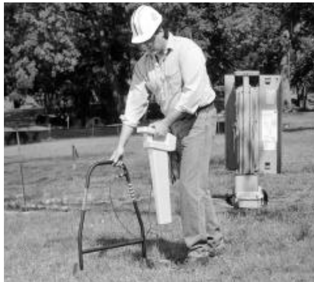
The Dynatel 2273 Cable/Fault Locator locates sheath (earth return) faults. 3
