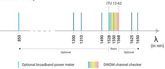
Channel checker and power meter wavelength range
