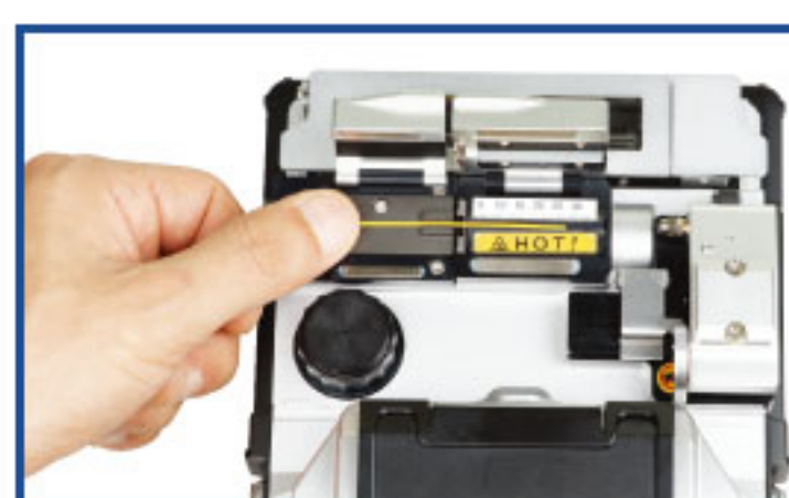
Stripping (No Cracks on Fiber)
