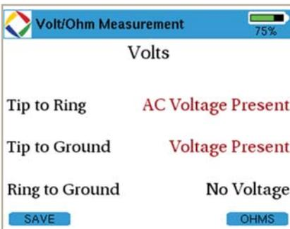
The Volt/Ohm mode indicates AC and DC voltages
