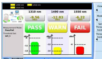
PON power meter screen
