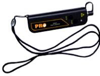
The VFL-5 is a compact but powerful visable light source with an output power up to 1mw. The VFL-5 can be used to locate sharp bends and breaks in jacketed or bare fiber. It can also be used to identify connectors in patch panels or indentify fibers during splicing operations.
