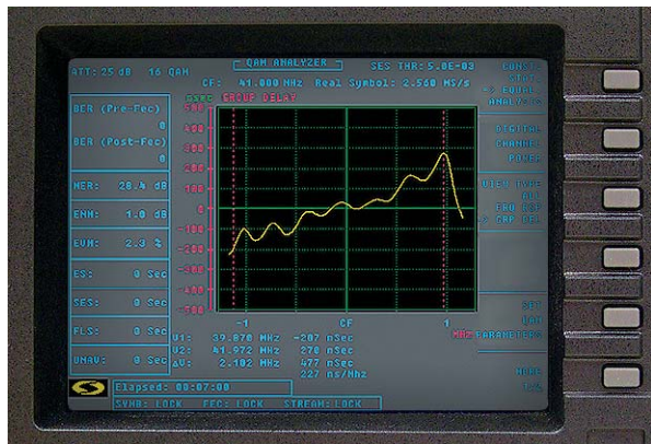
Zoomed Group Delay screen with \Delta nsec per MHz measurements
