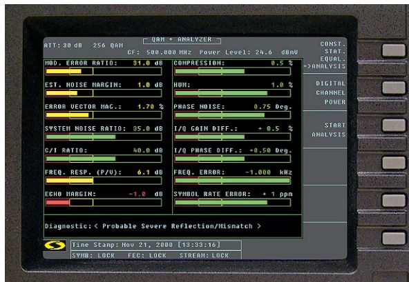
QAM Impairment Analysis (QIA) displays 14 performance measurements on one screen
