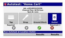
Multi-user support allows technicians that work in various territories to easily switch channel plans, standardized autotest apps, and test limits or login as a completely different user. The built-in web browser allows techs to upload job data in near real-time as well as transmit and receive channel plans, autotests, work orders, and firmware.
