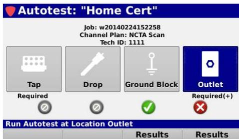
Multi-user support allows technicians that work in various territories to easily switch channel plans, standardized autotest apps, and test limits or login as a completely different user. The built-in web browser allows techs to upload job data in near real-time as well as transmit and receive channel plans, autotests, work orders and firmware.
